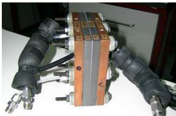
Fig. 6 - 25\text{ cm}^2 single cell and experimental set up.
